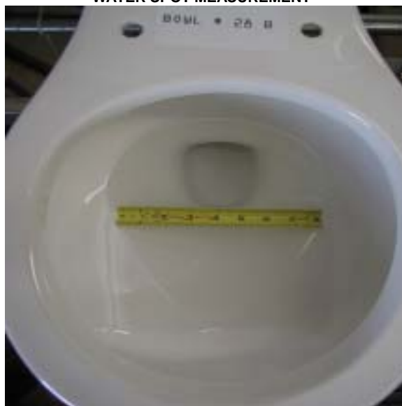
FIGURE 5 WATER SPOT MEASUREMENT
