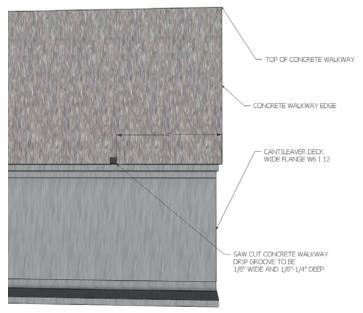
Figure 10: Drip Edge Detail (Section Cut)
