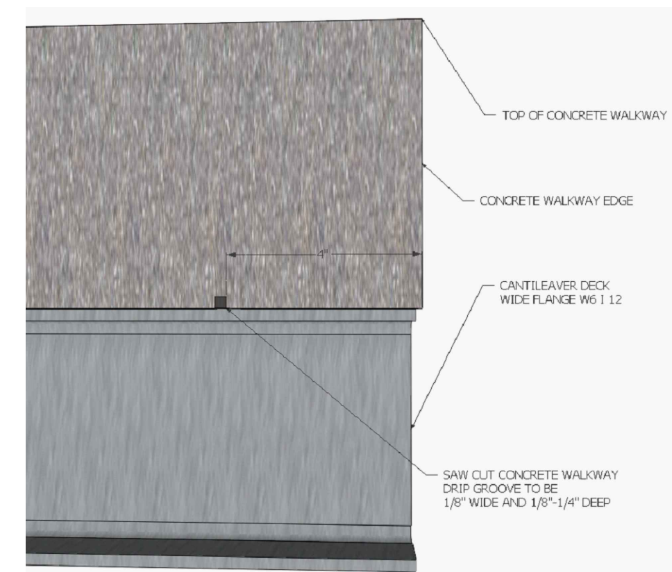
DRIP EDGE DETAIL (SECTION CUT)
