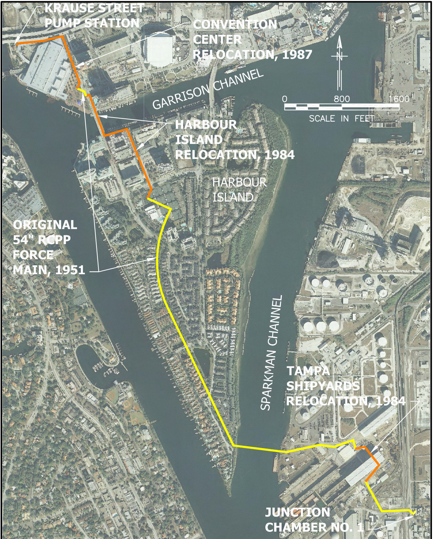
FIGURE 2 RELOCATIONS AND CURRENT FORCE MAIN CONFIGURATION
