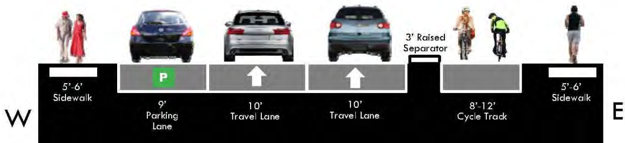
Phase 3c - 15th Street from 13th Avenue to 21st Avenue Proposed Typical Section
