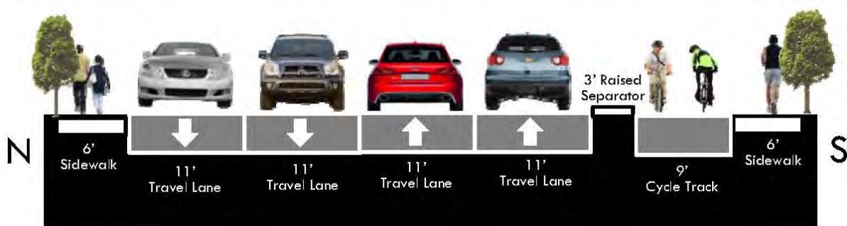
Phase 2b - Cass Street from Willow Avenue to Cass Street Bridge Proposed Typical Section
