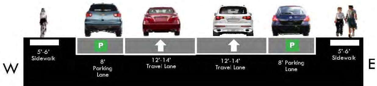
Phase 3c - 15th Street from 13th Avenue to 21st Avenue Existing Typical Section
