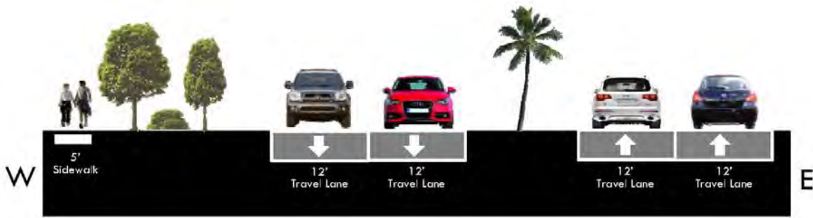
Phase 3a - Nuccio Parkway from Nebraska Avenue to 7th Avenue Existing Typical Section
