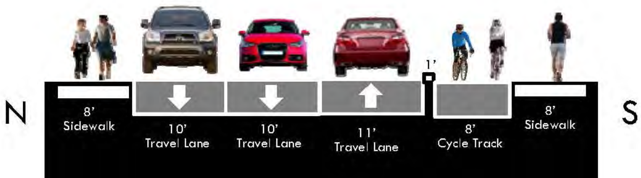
Phase 2b - Cass Street from Willow Avenue to Cass Street Bridge (Bridge Approach) Proposed Typical Section
