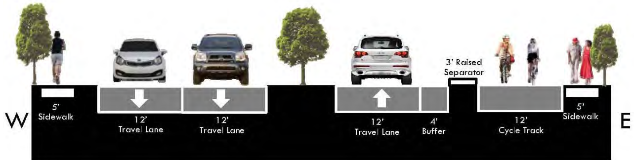
Phase 3b - Nuccio Parkway from 7th Avenue to 13th Avenue Proposed Typical Section
