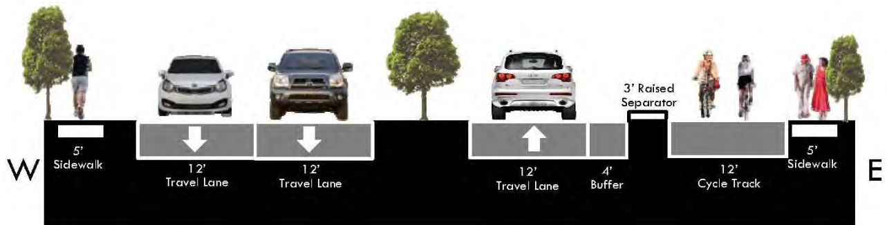
Phase 3b - Nuccio Parkway from 7th Avenue to 13th Avenue Proposed Typical Section
