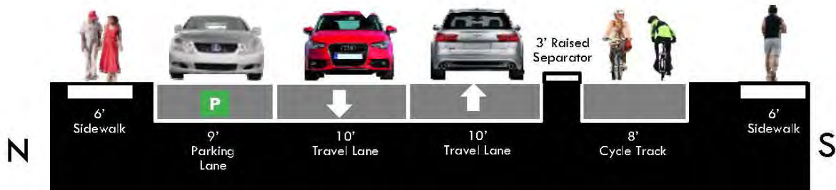
Phase 2a - Cass Street from Howard Avenue to Willow Avenue Proposed Typical Section
