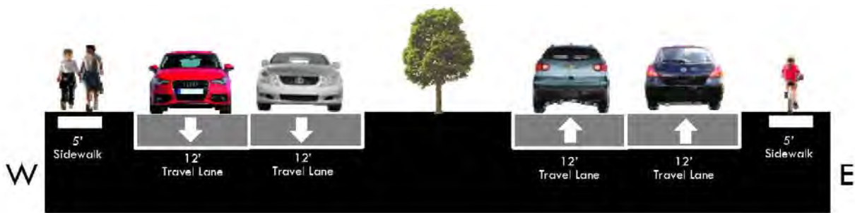
Phase 3b - Nuccio Parkway from 7th Avenue to 13th Avenue Existing Typical Section
