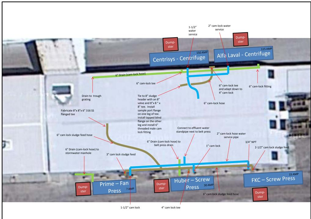
Figure 2-1: Equipment Locations and Connections for Round 1 Testing
