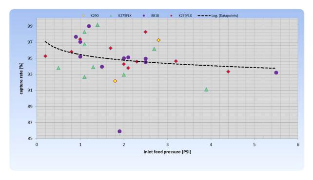
The pressure at the inlet flange applied to the feed also has a significant effect on the capture rate as shown in Figure 10 above. The pressure ratings exceeding approximately 2.5 psi caused the capture rate to decrease below an acceptable level.
