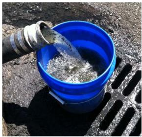
**Photo 4: Pressate from Screw Press**
