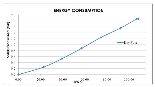
Figure 5: Solids Processed vs. Energy
