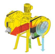
rotation/friction of the filter screens continuously moves the cake solids pass the restrictor arm to be discharged for disposal or further processing. Operation of the Rotary Fan
