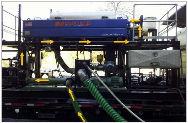
Figure3: Sludge Feed Flow
