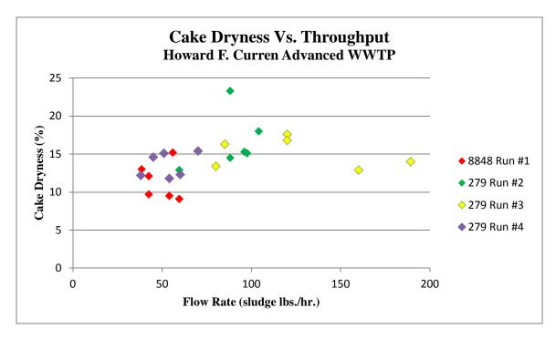
The dewatering rate is scalable by using the hydraulic throughput (listed in gpm) per square foot of screen area by the square foot of filtration area per dewatering channel of each of the Rotary Fan Press sizes listed:
