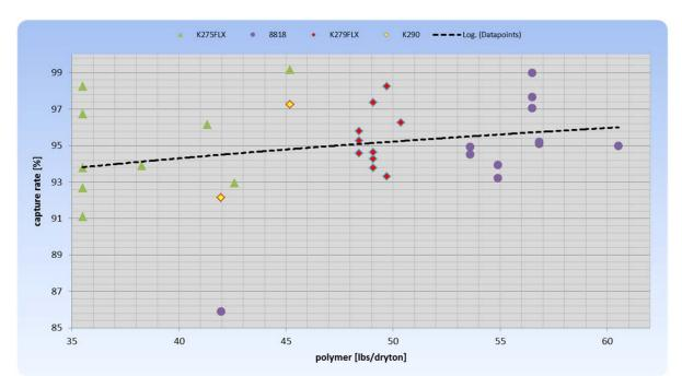
FIGURE 8 – POLYMER CONSUMPTION AND CAPTURE RATE
