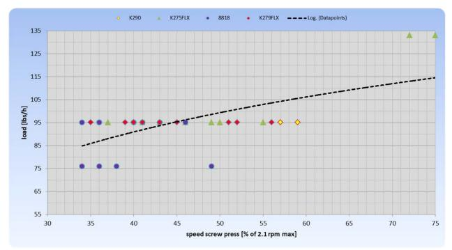
FIGURE 5 – SCREW SPEED EFFECT ON THROUGHPUT
