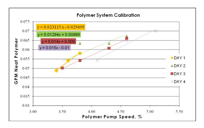
Figure 1: Daily Polymer Pump Dose Calibration
