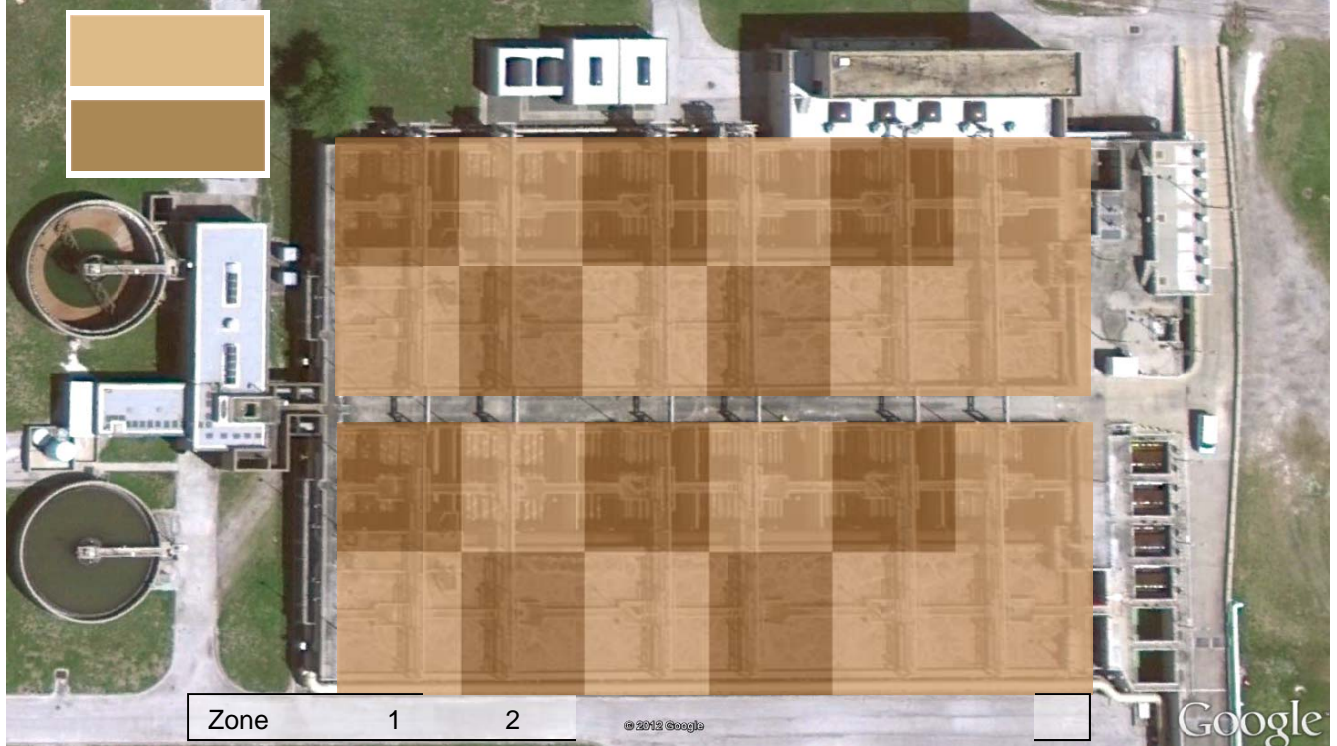
Figure 5 Alternative 2 On/Off Aeration Strategy
