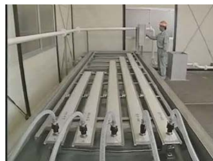
Figure 4. Each individual AEROSTRIP diffuser is factory-tested
