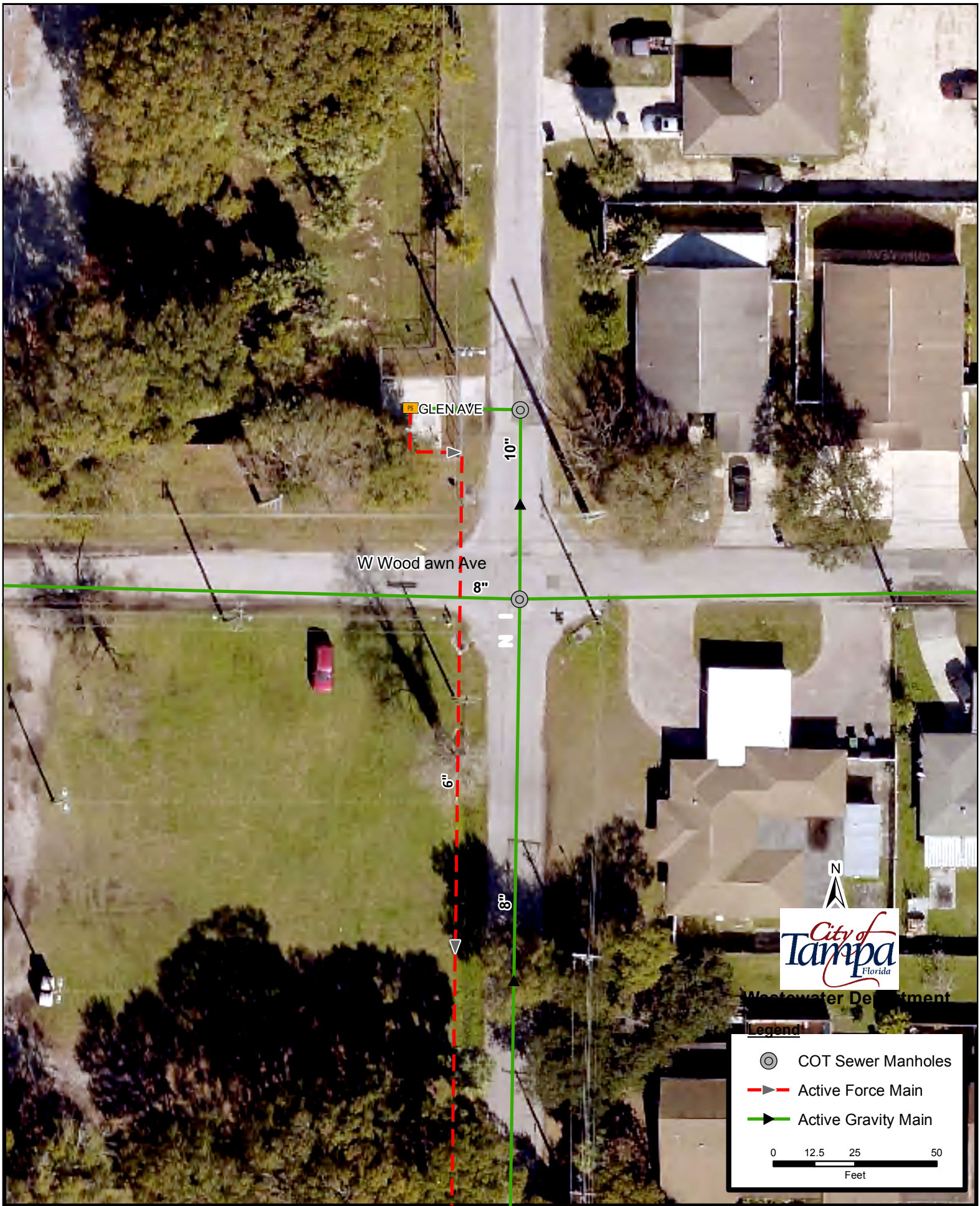
Exhibit No. 28 - Glen Avenue Pumping Station
